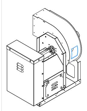
Provides easy inspection or cleaning of the fan interior and wheel
